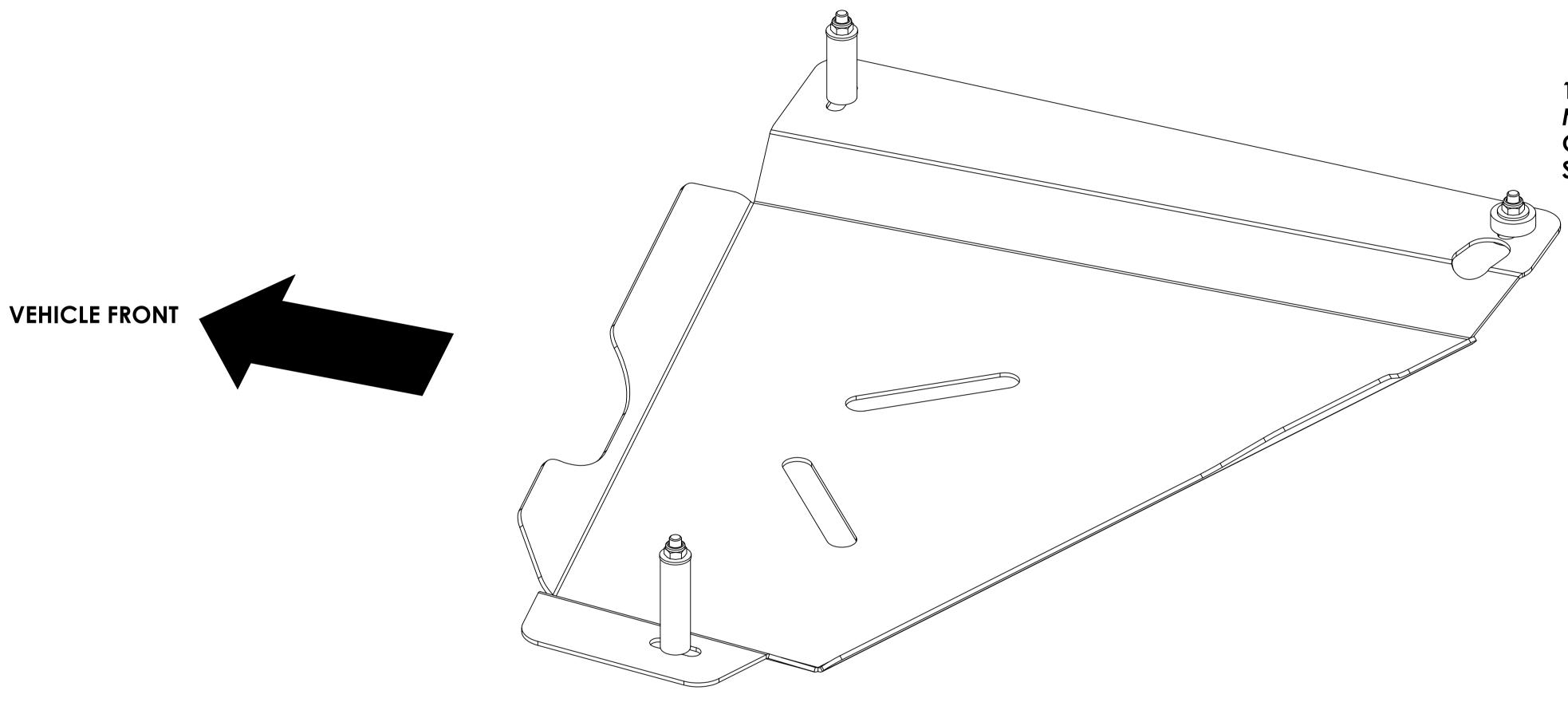
10mm SPACER BETWEEN PLATE & CHASSIS M8x30 & LARGE MUDGUARD WASHER ON PLATE SIDE SMALLER FLAT WASHER & NYLOC INSIDE
